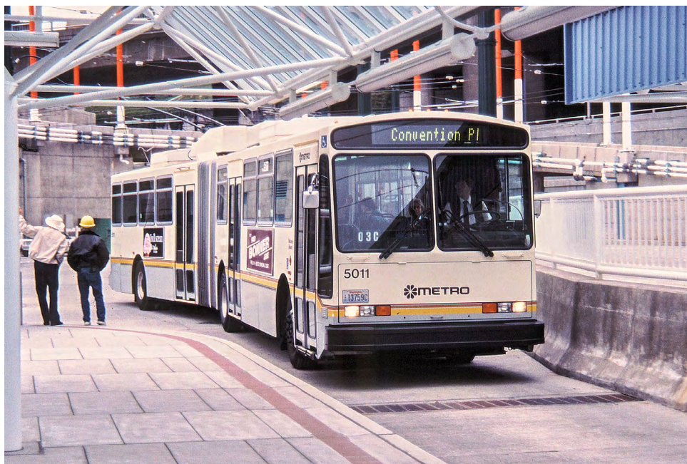
Above: Seattle's Bredas had a diesel drive to the back axle with the electric drive operating on the centre axle. 5011 is seen on the tunnel opening day.
